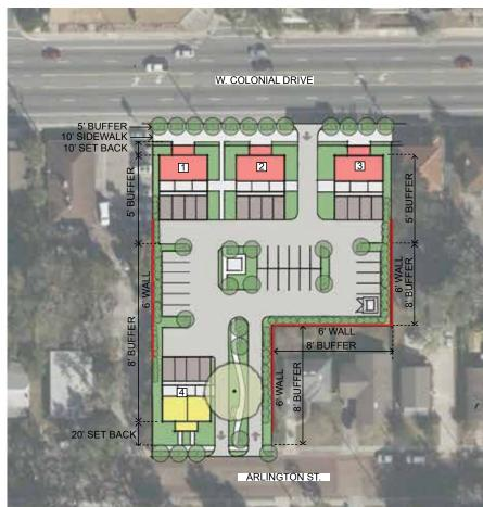
Figure 5 illustrates the proposed site plan for the redevelopment on Site 2: 744 **West Colonial Drive.**
