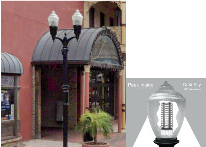
Pedestrian Light Retrofit the existing double acorn lights with a dark-sky compliant cutoff feature for the bulbs. The luminaire is the Granville, and the pole is the Wadsworth Black with base from the Orlando Utility Commission (OUC).
