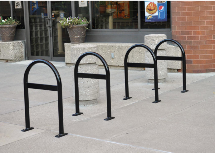
Bike Rack The surface-mounted Thomas Steele U24 Bike Rack with a lean bar in a black powdercoated finish, or similar, should be used.
