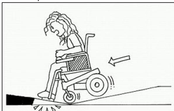
Steep counter slopes will cause some wheelchairs to catch on back rollers and lose drive wheel traction. For others, the steep counter slope will catch footrests.
