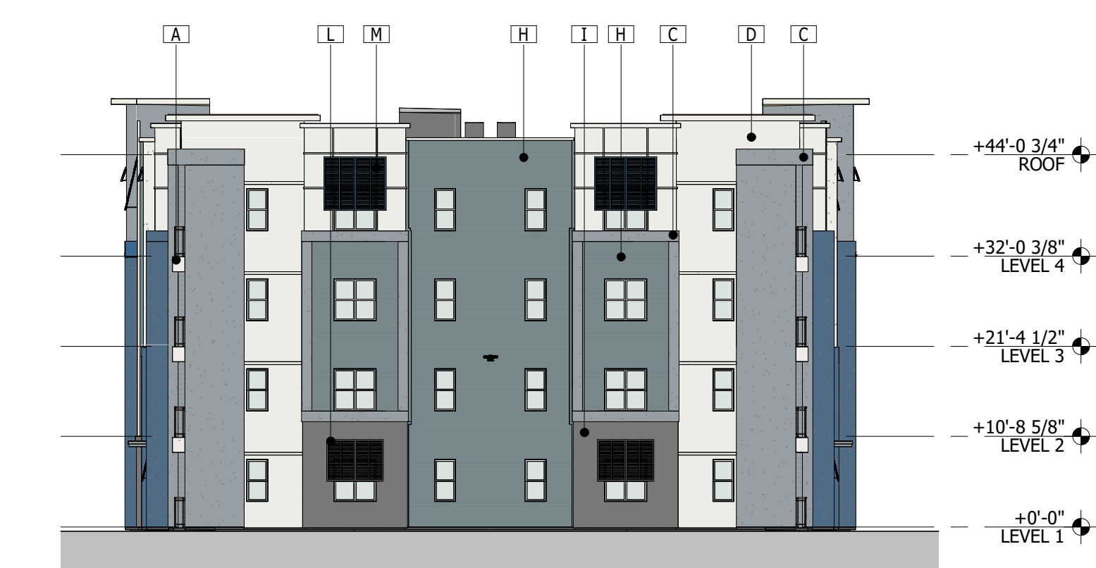
3 BLDG TYPE III - LEFT ELEVATION SCALE: 1/16" = 1'-0"
