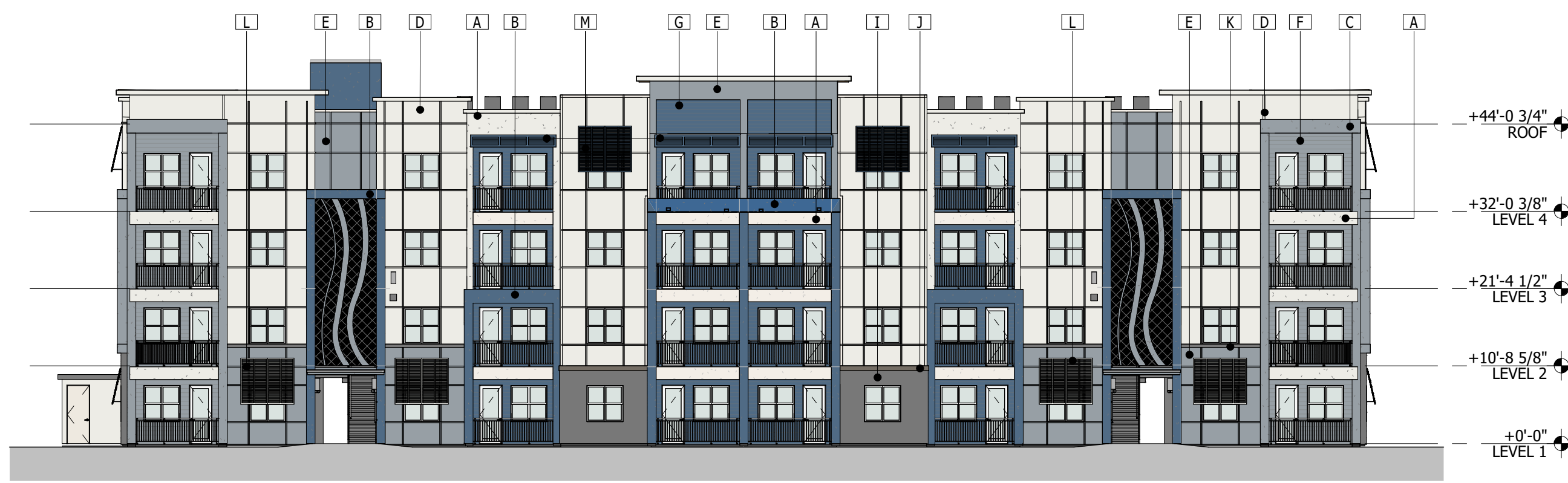
4 BLDG TYPE III - REAR ELEVATION SCALE: 1/16" = 1'-0"
